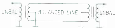
Figure 3. The use of a transformer for the conversion of a line to and from unbalanced to balanced.
