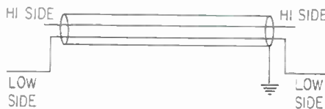
Figure 4. A shielded unbalanced line using a double conductor within a shielded shell.
